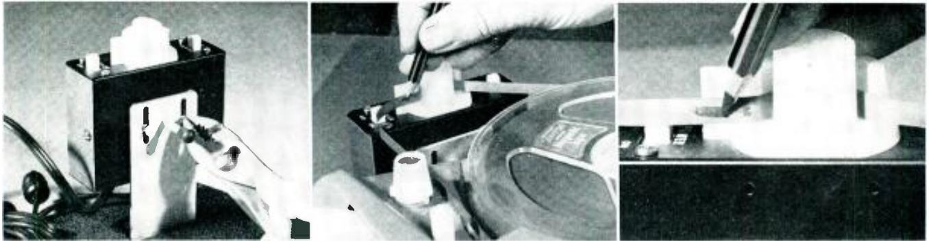
Left: the height is adjusted by means of two screws and a slotted metal strip. The adjustments provided will cover most recorders. Center: the cue for a slide change is marked on the oxide side of the tape using a special pencil supplied with the unit. Right: close-up shows width and length of pencil mark. A few seconds must be allowed to elapse between slide changes.
