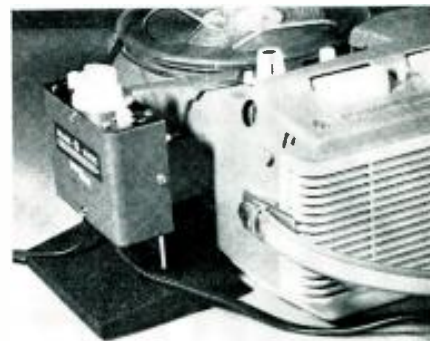
The unit set up on the feed reel side of a recorder. The head should be positioned so that the tape moves evenly from the reel to the tape head slot.
